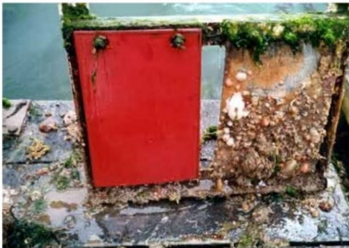
Figure 5: Evidence of the antifouling effect of tributyltin (TBT): absence of biofouling on the left panel, painted with TBT-based antifouling; accentuated biofouling on an unpainted panel, on the right.
